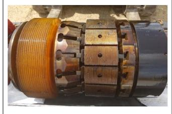
Once the grips have connected with the pipe, the axial force of the tool extrudes the urethane sealing element until it creates a bubble tight seal against the pipe wall.
