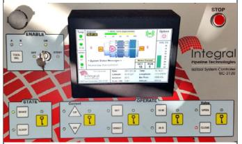
The tool ran through its complete cycle and sent a confirmation that the set current had been reached and the tool was set in 47 minutes. The internal bypass in the US IsoTool was closed and the pressure DS of the tool was dropped and the 30 minute Isolation Assurance Test was performed.
